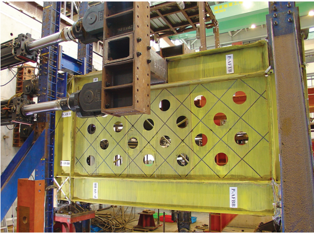
Fig. 9. Perforated panel specimen (P) before testing.
